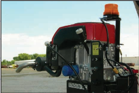
Honda 20.8 H.P. electric start air cooled gasoline engine.
