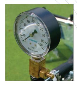
A LARGE PRESSURE GAUGE is easy to view your proper spray pressure setting and a needle value is standard to dampen gauge needle pulsation and vibration.
