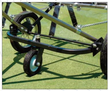
THIRD WHEEL KIT allows user to maintain proper tip height for a uniform application rate. This optional kit will retrofit all Broyhill walking booms. Order I-2679
