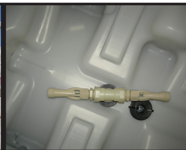
Dual jet agitation on 40 gal unit
