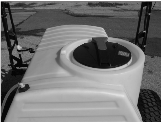
Drain plug in fillwell trough routes spilled chemicals back to spray tank.
