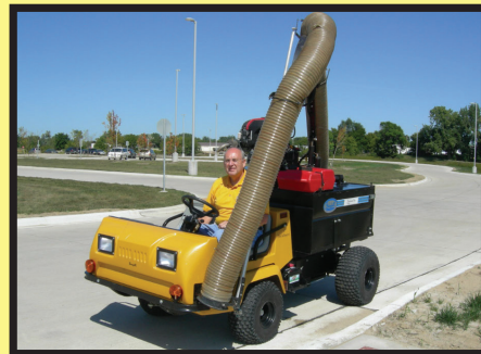
Stadium vac unit shown here cleaning up industrial park street litter.
