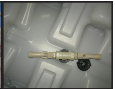
Dual jet agitation on 40 gal unit
