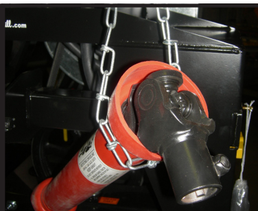
PTO Shaft Chain Hanger (when not in use) is standard equipment.
